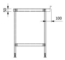
UNDERTOP ------- 1.2mm Thick Galvanised Steel UNDERSHELF (If Applicable) -- 1mm Thick 430 Grade St/Steel, 43mm Turndowns LEGS --- 30x30mm 430 Grade St/Steel Tie Bars (If Applicable)-30x30/15/5mm 430 Grade St/Steel PANELS (If Applicable) ---------- 0.7mm Thick 430 Grade St/Steel
