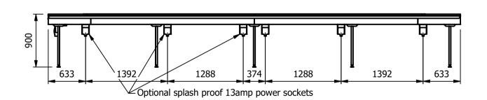
Emergency-stop button at each end. Speed adjustable from 0 to 12 metres/minute Maintenance-free drum motor
