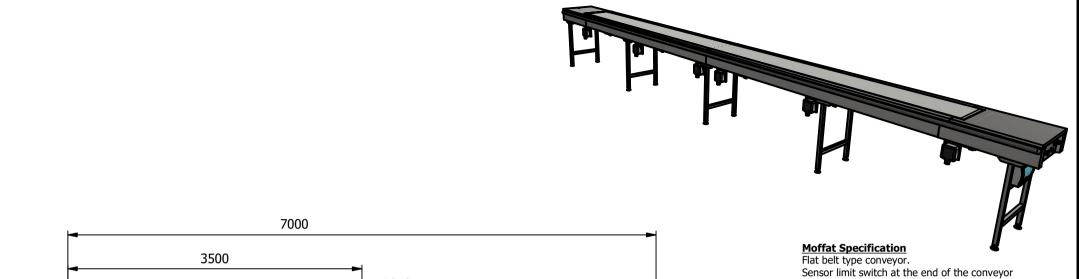
5858 Direction ►► Full length bumper Photo electric sensor on both sides automatically prevents trays clashing.
