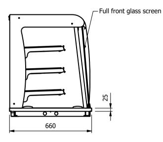
ALL DIMENSIONS IN (mm), TOLERANCE = LINEAR ± 0.5mm, ANGULAR ± 0.5mm (OR AS STATED). ALL SHARP EDGES TO BE REMOVED FROM SHEET METAL PARTS
