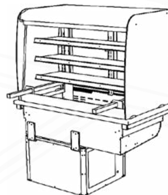
Lifting Plate Temporarily fit to each corner of the well
