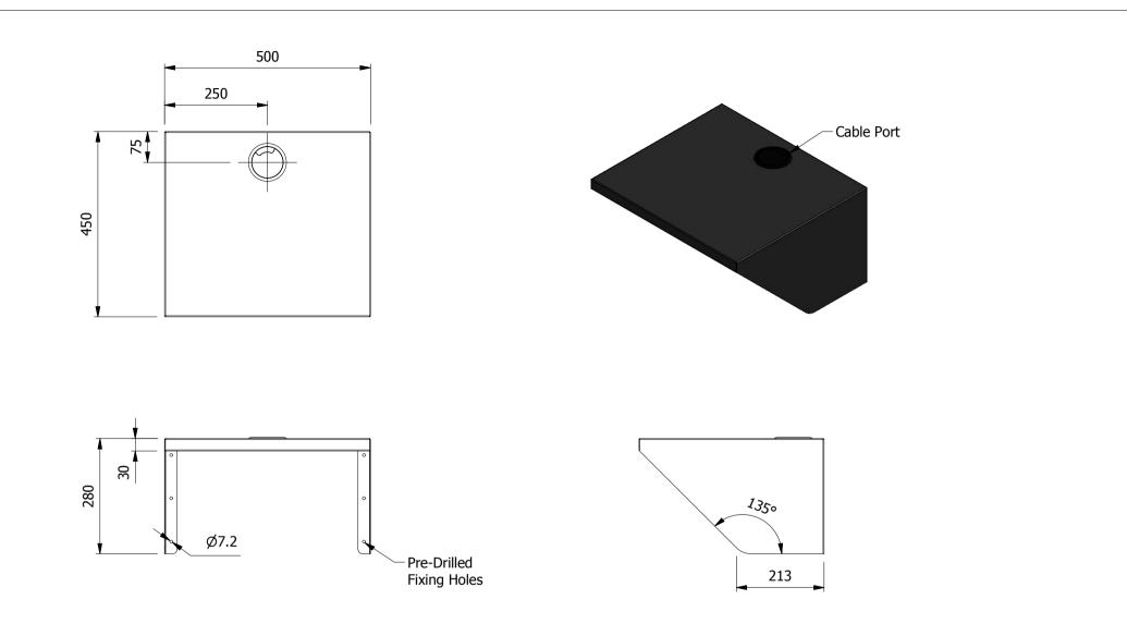
Moffat Specification SWS TOP ------1.5mm Thick 304 Grade St/Steel
